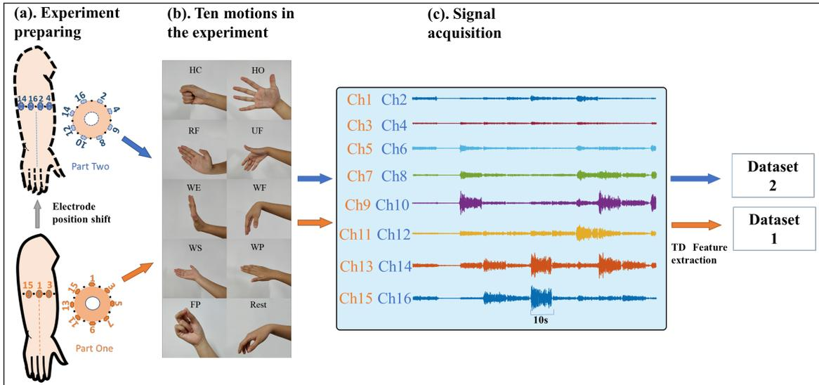
Fig 1. Acquisition schematic of EMG with 8-channel bipolar differential EMG sensor electrodes.
