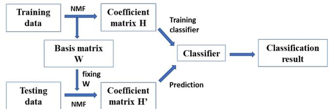
Fig 1. Flowchart of pattern recognition based on NMF and LDA.
