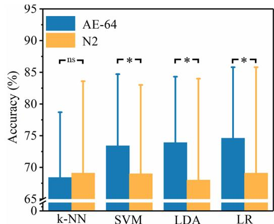
Fig. 2. Comparisons of classification accuracies between AE-64 and N2 for 4 different classifiers. “AE-64” represents 64-dimensional features encoded using the AE model, and “N2” represents N2 amplitude features of all 62 channels. Four classifiers, k-NN (k = 3), SVM (linear kernel), LDA, LR
