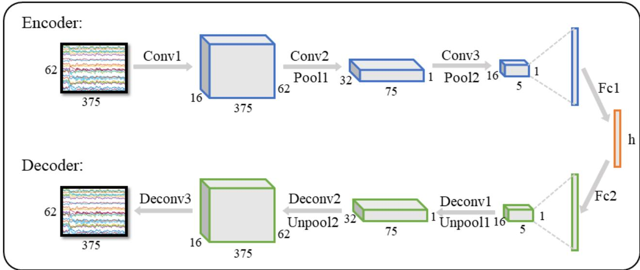
Fig. 1. The proposed AE model based on EEGNet [14].
