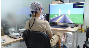
Fig. 1: The virtual environment of non-emergency task. Subjects sit on the chair with right foot on the brake pedal and take actions according to what they saw on the screen in front of them. In this virtual environment, it displays a suburban road, with no traffic signs or traffic lights. The setting of the virtual environment is different between emergency and non-emergency tasks.
